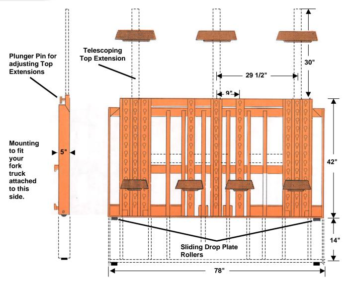
The model 4278 is designed to "Top Handle" products as triples and quads depending upon product size. Highway trailers can be loaded in minimum amount of time by loading the width of a trailer in one trip.
